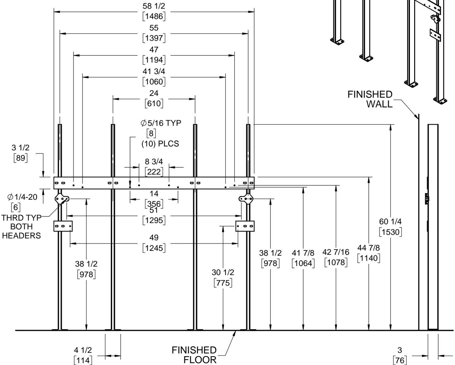
JOSAM RECOMMENDS - FEET BE SECURED TO FLOOR WITH 1/2" BOLTS AND ANCHORS BY OTHERS
