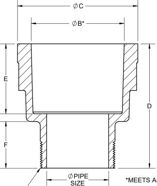
\*MEETS ASTM A-47 XH CAST IRON SOIL PIPE STANDARD
